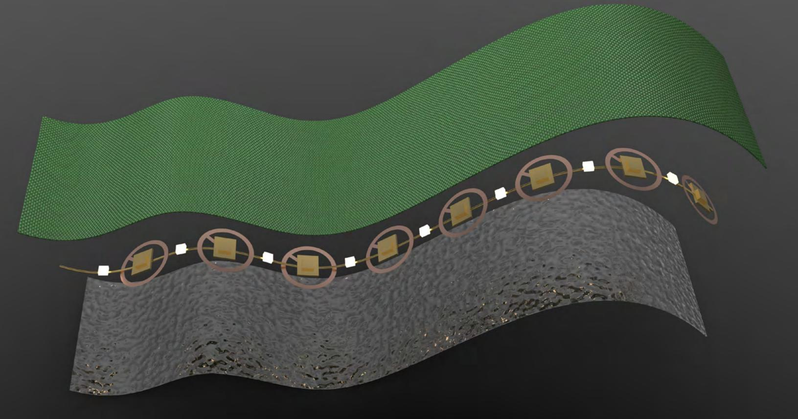
Minder tapes contain a combination of vibration micro-motors, LEDS, heat-producing coils, and constricting wires paired with Bluetooth transponders and micro PCBs to produce light, heat, vibration and
