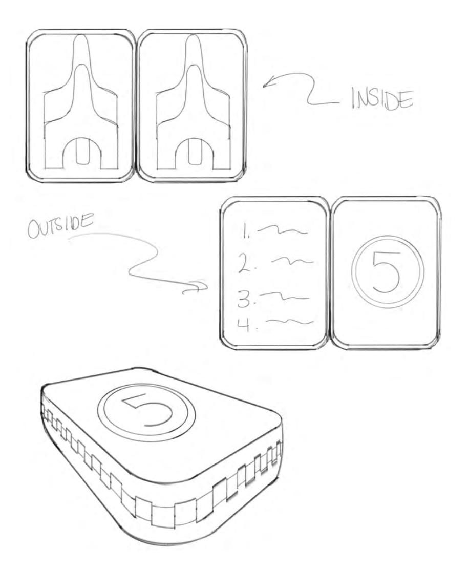
These sketches explore options such as a case for Narcan that includes a timer and a re-imagined color-changing body for the applicator itself. A **separate, small, attachable timer** was chosen for its feasibility and ease of production.
