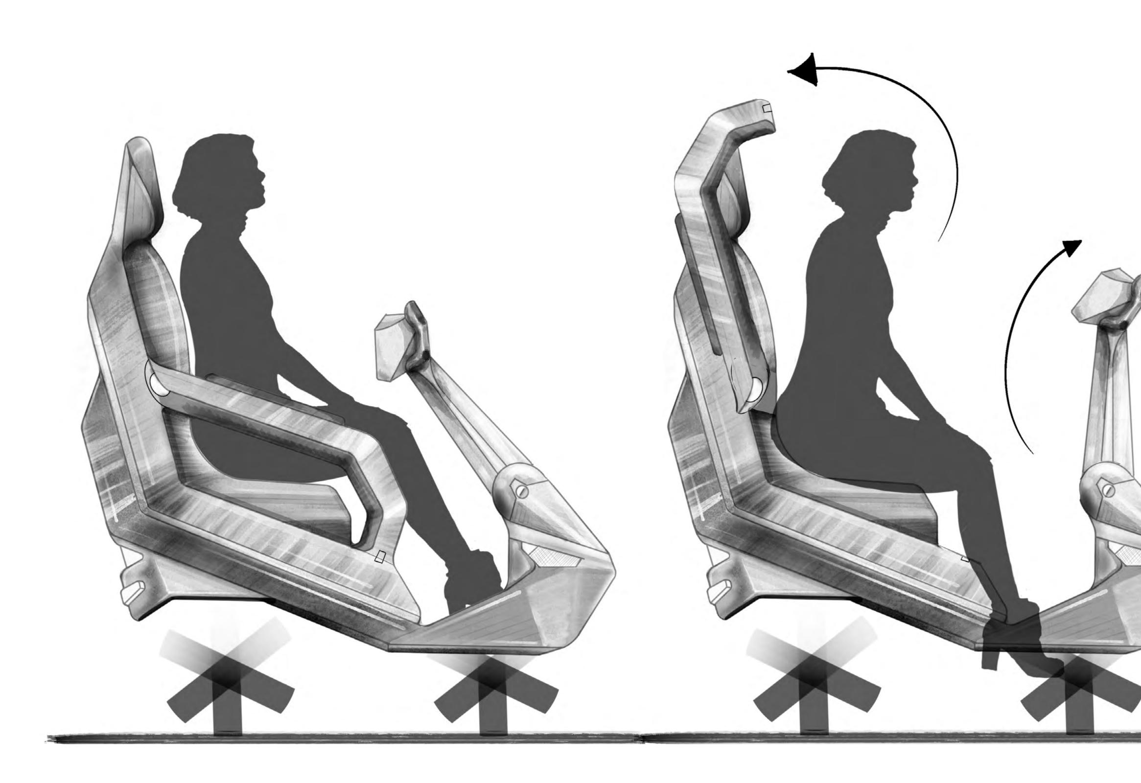
The arms and steering column of the Pascal scooter pivot upwards to allow easy entry and exit from the vehicle, especially for those that move from the scooter to a wheelchair or other mobilityassisting device. When not lifted, these elements securely lock in place to prevent a user from accidentally falling out during turns or when navigating rougher terrain.
