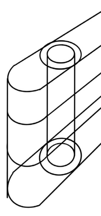
A bulkier folding hinge was chosen due to the strength necessary to maintain stability under pressure Brass hinges with a thick, hollow structure are both stable and can fit into the existing tenons cut for hinge plates, increasing adoption and reducing expense for the resident
