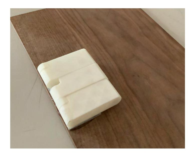
Proof of concept was achieved in **full scale** experimentation at Pratt Studios in Brooklyn. A fullsized, framed door was used to test the strength and form of a folding hinge with simple steel plates.
