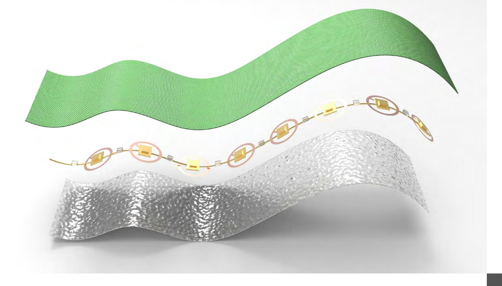
Each tape section contains these elements and a micro-battery that is powered by utilizing the natural electrolysis that occurs within human sweat (which is largely saline. Various versions of all these technologies are emerging now, but have all been proven to be feasible in a medical context.
